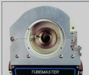
Collets removed to show Fillet Weld
