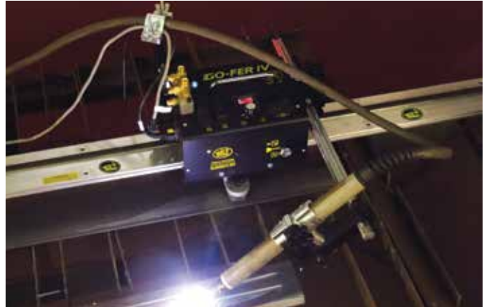
Shown above, plasma setup to perform back gouging
