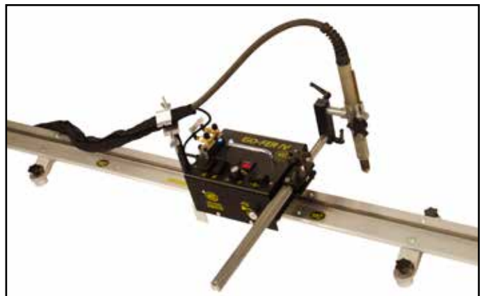
Shown above, plasma setup of Go-fer IV
